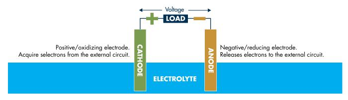
The medium that provides the ion transport mechanism between the cathode and anode of a cell.
