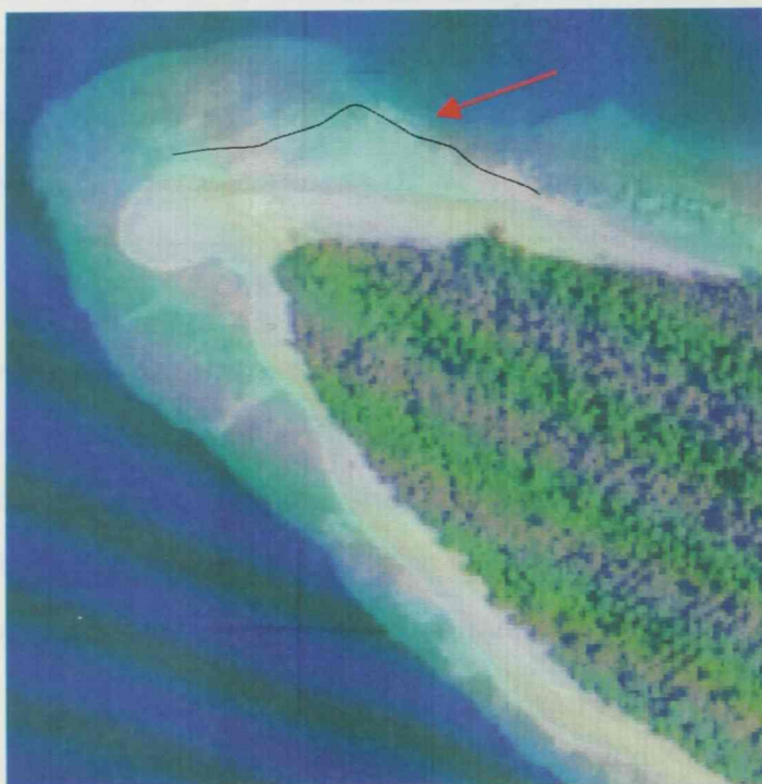
Figure 6.17 Sediment accumulation on the northwestern end of Maaddoo. The dotted line marks the position of sediment accumulation in the previous season, and the red arrow shows the point from where sediments were lost over the reef as shown in the previous figure (Figure 6.16).
