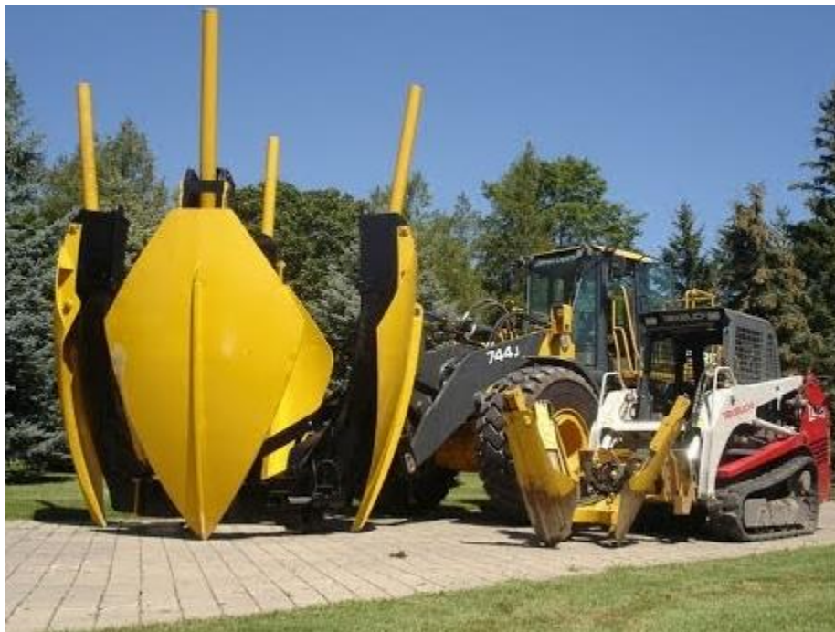
Figure 75: Automated spade used for removing trees
