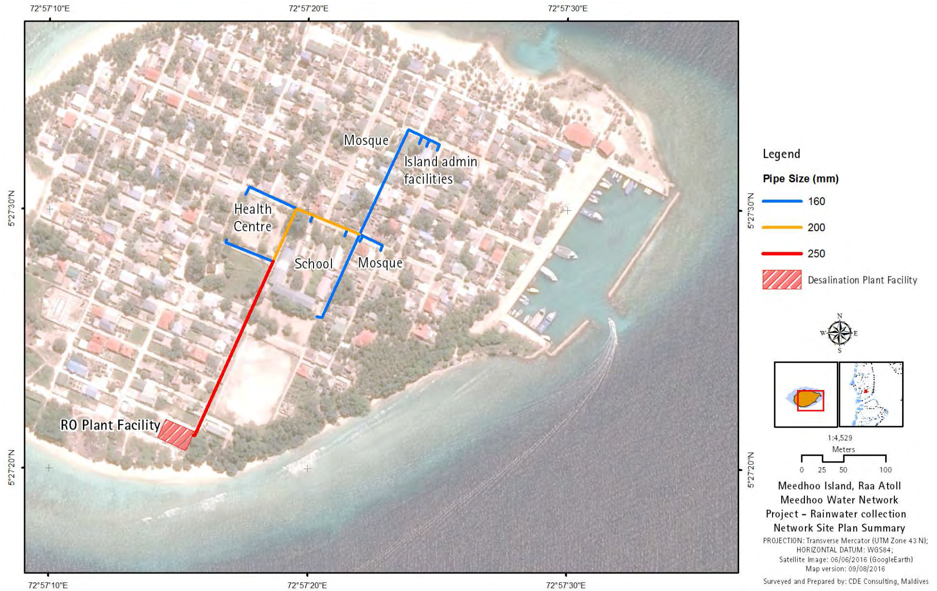
Figure 2.2: Project rainwater network site plan summary
