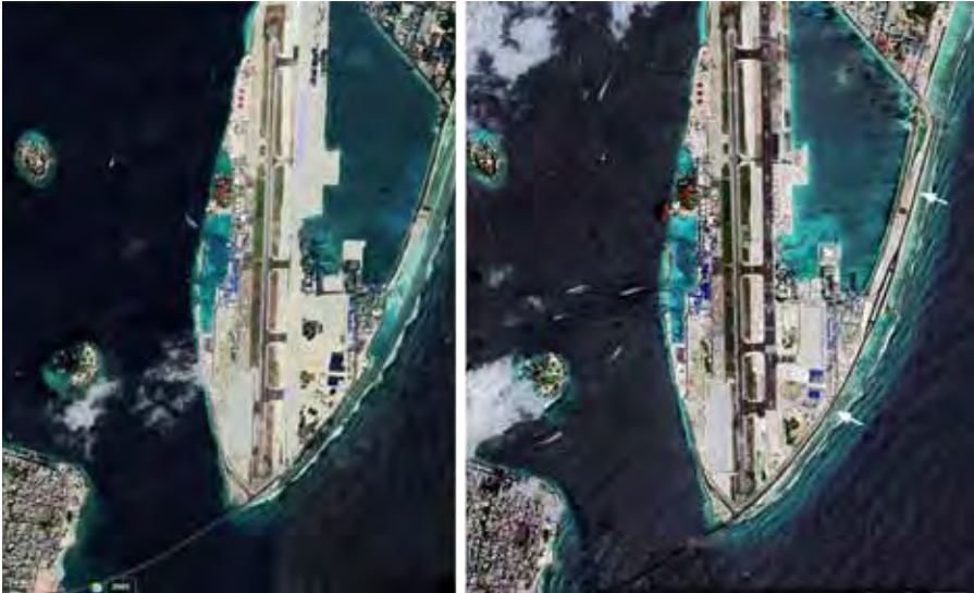
The photo above shows the link road from the bridge to Hulhumalé. The road is about 4 kilometres long and has four lanes. The road is just below the aircraft approach path to Hulhulé airport runway. Earlier there was a narrower road from the airport to Hulhumalé. The wider road required extensive reclamation.
