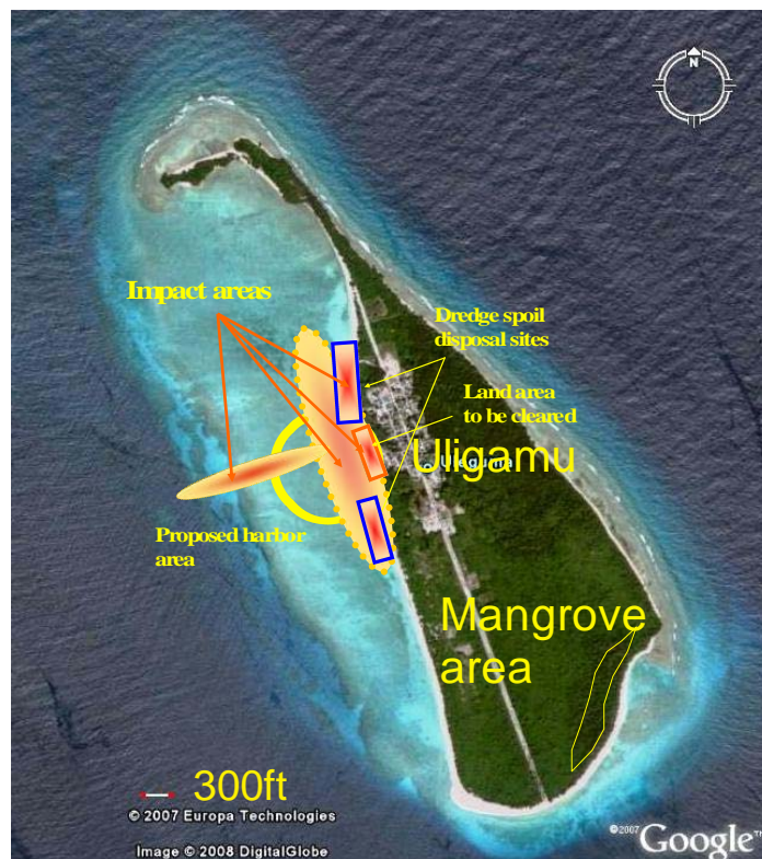
Figure 3: Project boundaries with possible direct and indirect impact areas. Dark red color represents direct impacts while the lighter color represents indirect impacts
