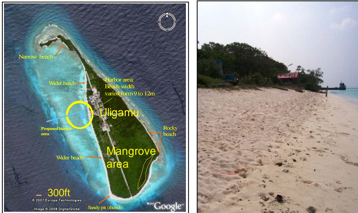
Figure 9: Beach widths of Uligamu (left). Wider beach was found at the southern side of harbor (right)
