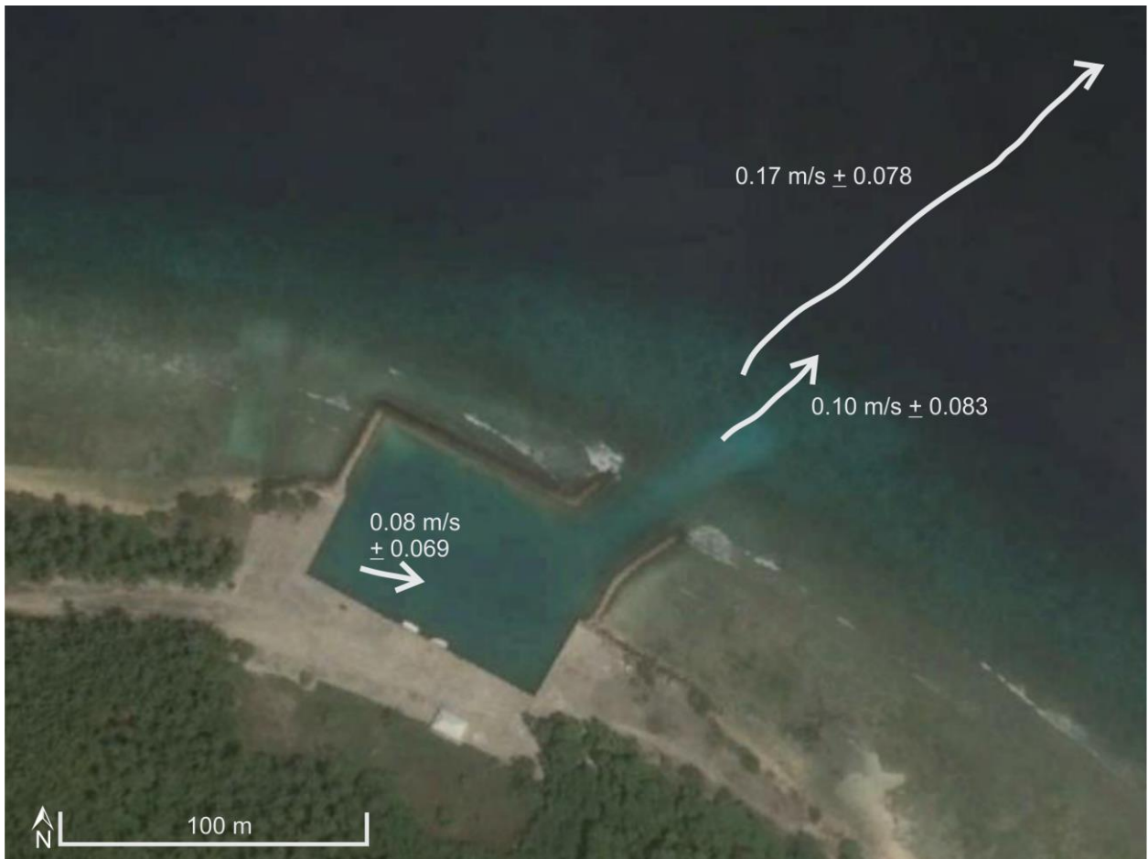
Figure 12. Ocean surface current speeds ( \text{ms}^{-1} ) in the channel, outside the channel and inside the harbour basin, as were observed on November 7, 2015.
