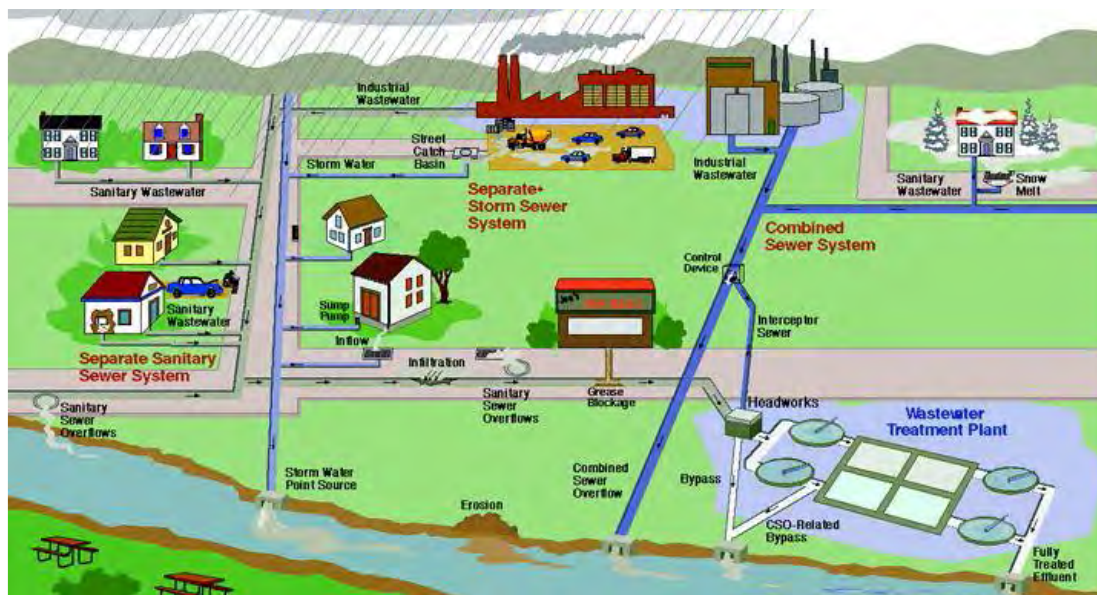
Figure 2.9: Components simulated in US-EPA SWMM (Storm Water Management Model) rainfall-runoff simulation model (Adapted from Source: SWMM User's Manual Version 5.1)
