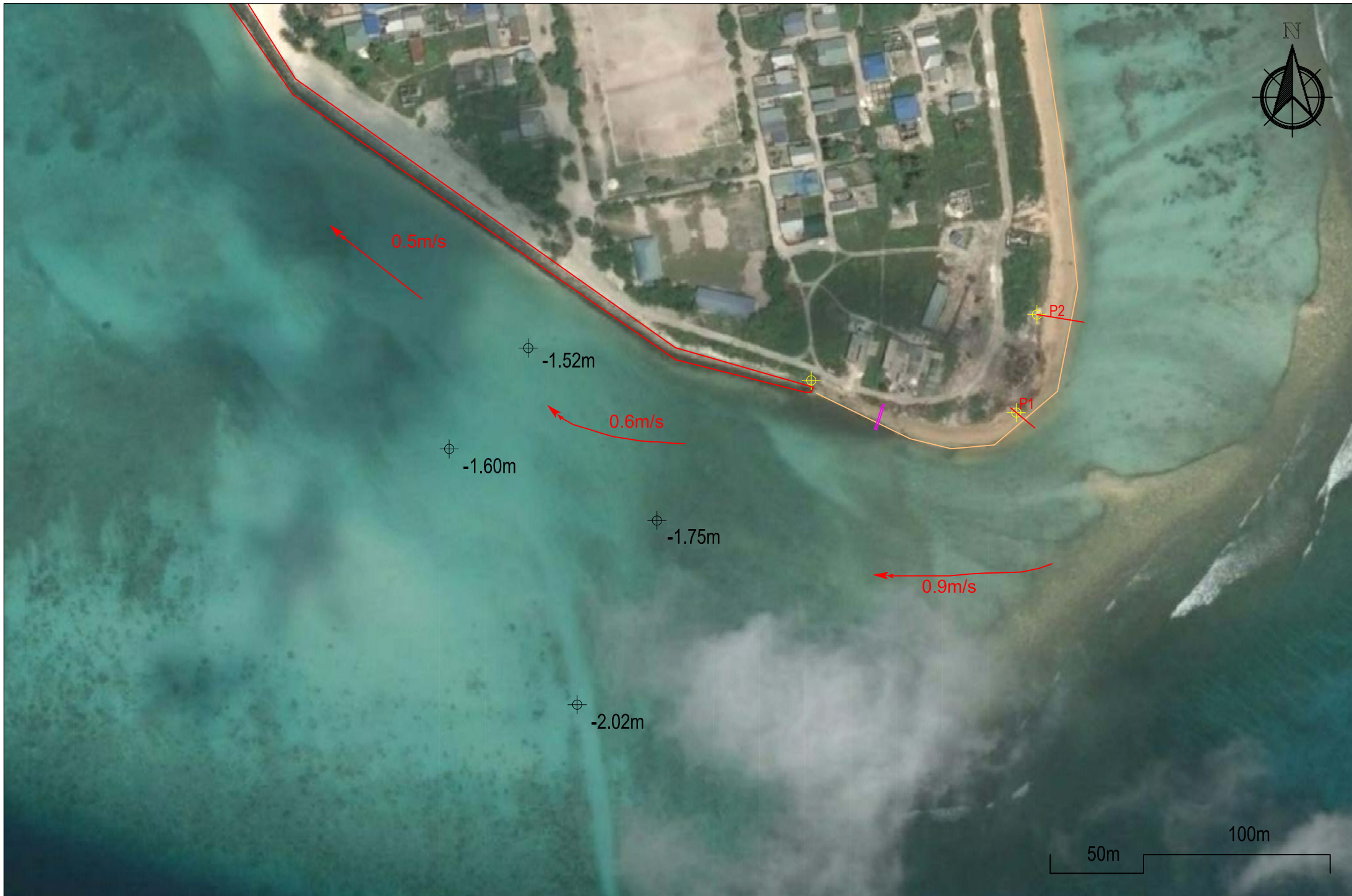
Figure 4-4: Bathymetry and drogue test results
