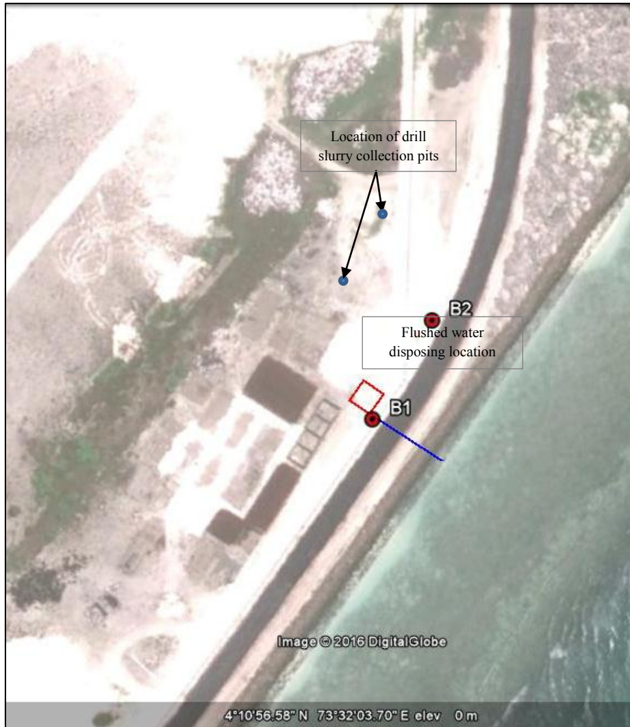
Figure 3 Locations of boreholes (B1, B2), drill slurry collection pits and flushed water disposal site
