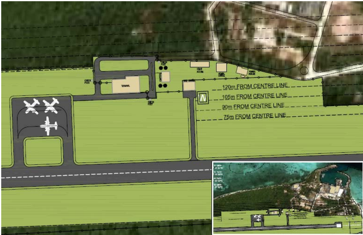
Figure 8: Layout of the reception terminal and the administrative and staff accommodation and power house building (inset to show the complete area including the arrival area)
