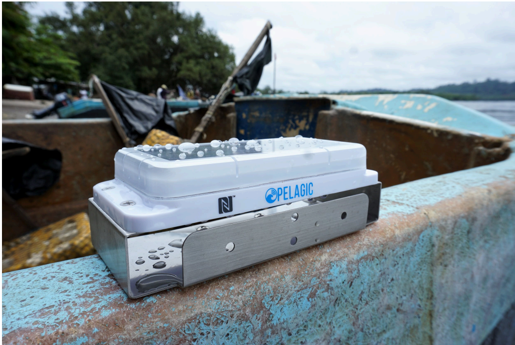
Figure 9. Pelagic Data Systems' solar-powered vessel tracking system (Pelagic Data Systems, 2019).
