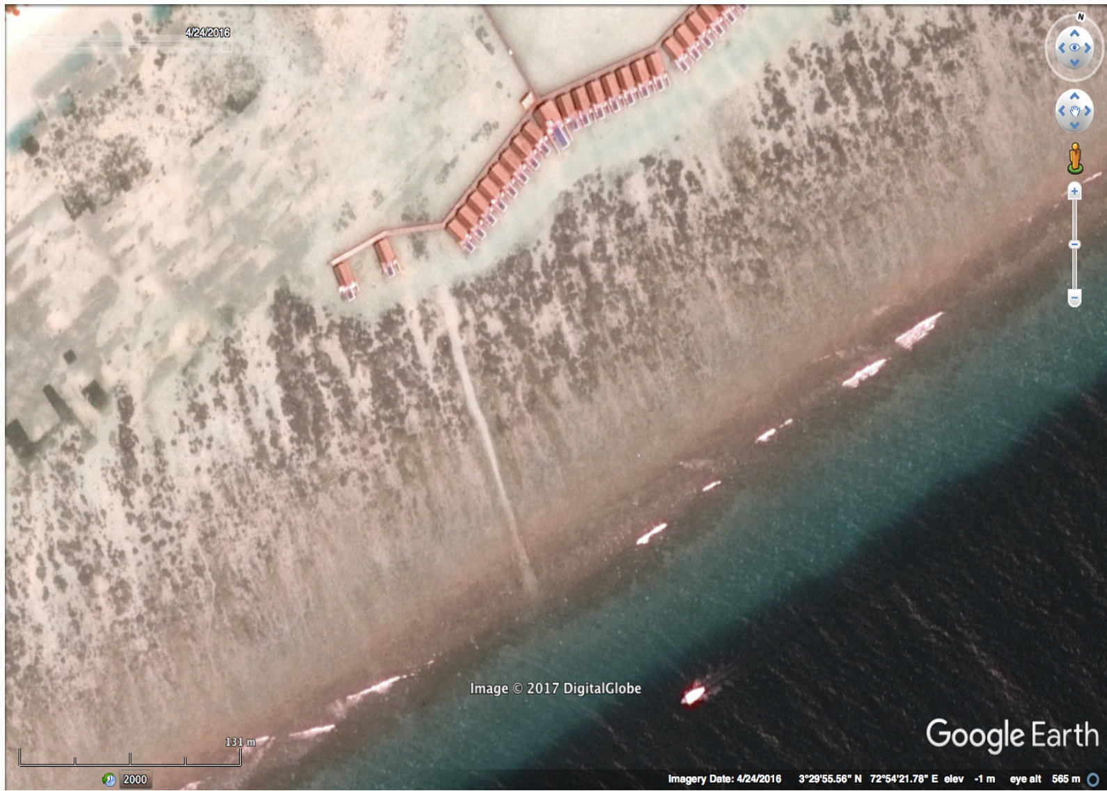
Figure 5.13: Google Earth Image of a boat channel dug by Lux resort on Dhidhoofinolhu Island.
