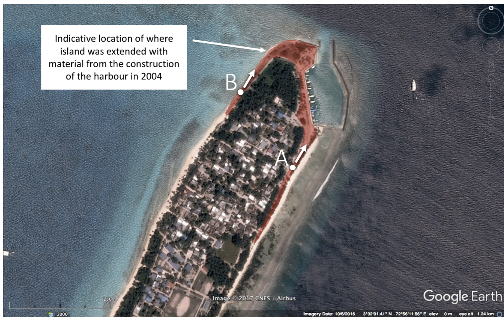
Figure 3.9: Harbour excavation material deposits. A and B refer to the location of photos shown in figures 3.10 and 3.11. Arrows next to A and B indicate the direction in which the photos were taken.
