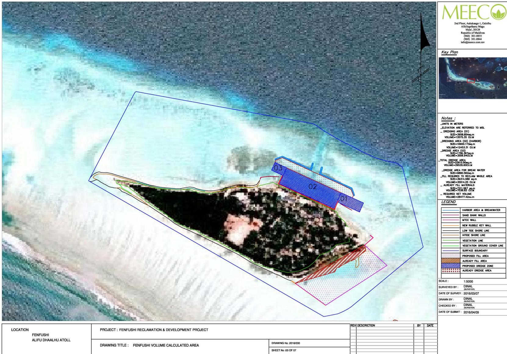
Figure 18: Size of dredge areas and amount of fill material available at proposed dredge zones 1,2 and 3.
