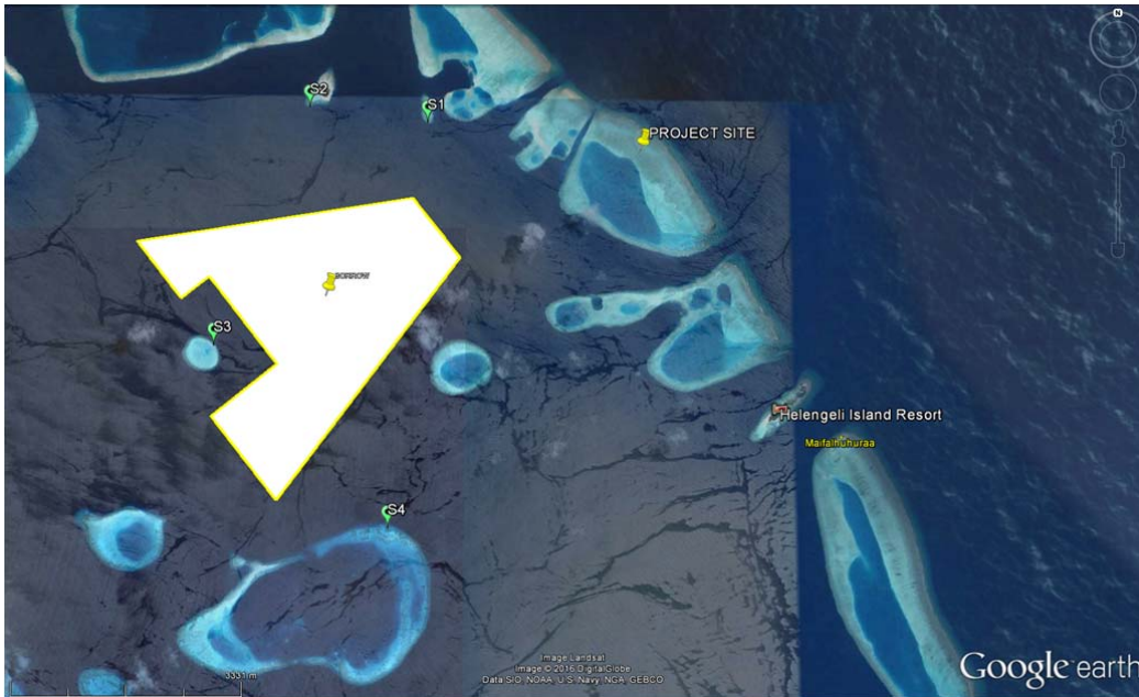
Figure 24 Proposed points for water quality monitoring at borrow area (S1, S2, S3, and S4)
