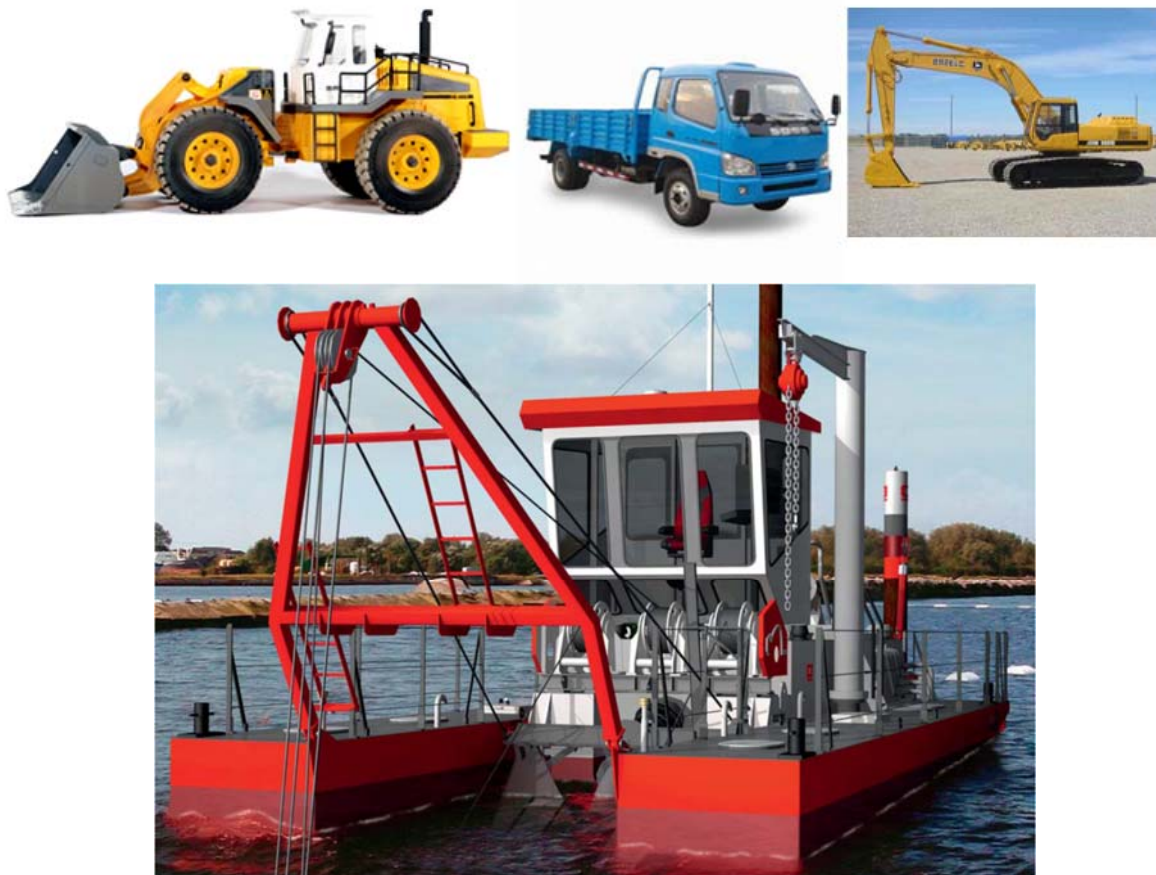
Figure 4: Typical heavy machinery and equipment that will be used for resort construction, dredging and reclamation, IHC Beaver® series cutter suction dredger (bottom).
