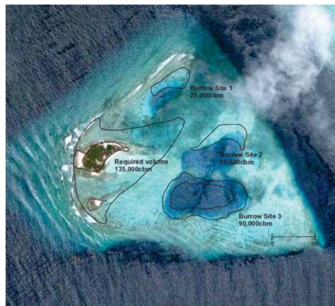
Figure 5: Akirifushi Falhu showing location of sand burrow areas and quantity of sand burrowed from each area and proposed land reclamation and total quantity of sand required
