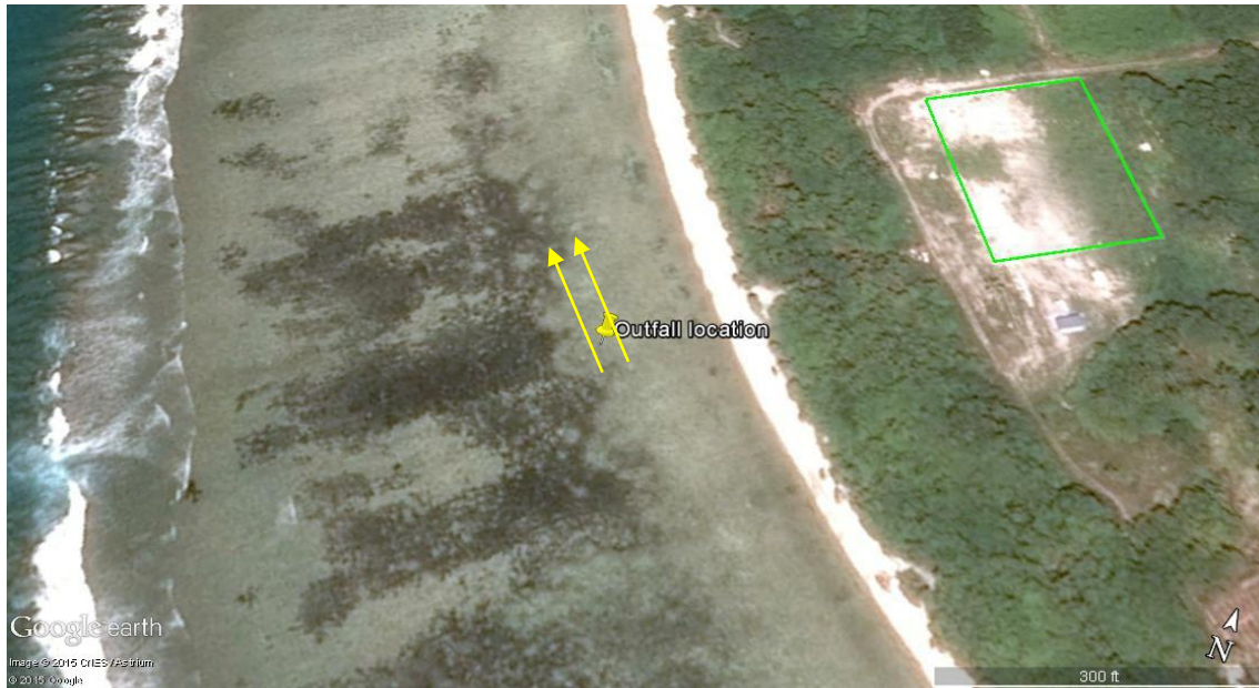
Figure 13. Current direction at the effluent outfall location indicated by yellow lines.
