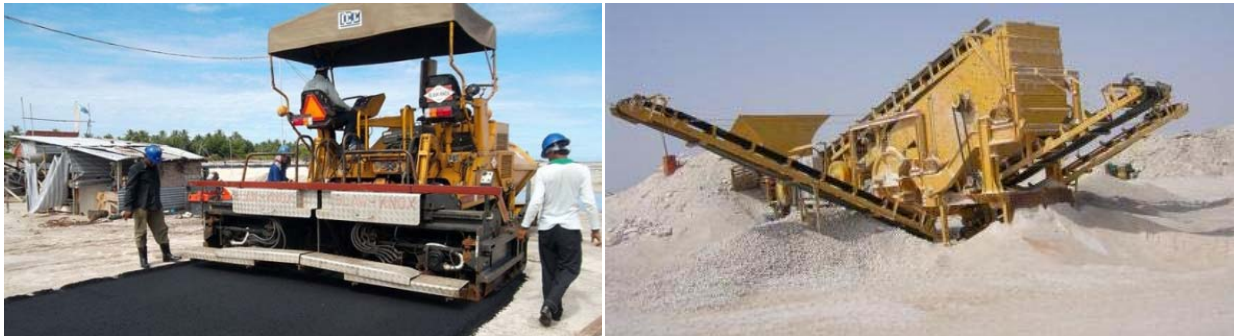
Figure 3: Some of the heavy machinery that will have to be used for the construction work and that would require to be deployed to Kooddoo Island. Asphalt paving machine (left), Jaw-crusher (right)
