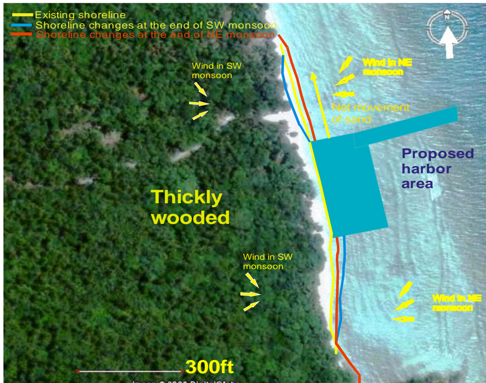
Figure 15: Possible alteration of shoreline as a result of harbor construction
