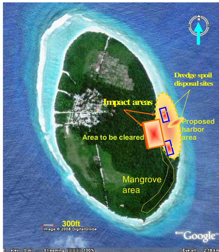
Figure 4: Project boundaries with possible direct and indirect impact areas. Dark red color represents direct impacts while the lighter color represents indirect impacts
