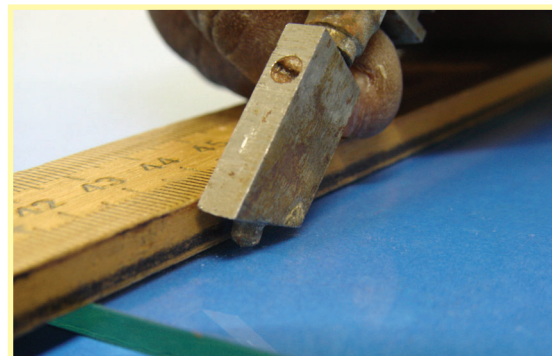
A tiny diamond at the tip is used to scratch the glass.
