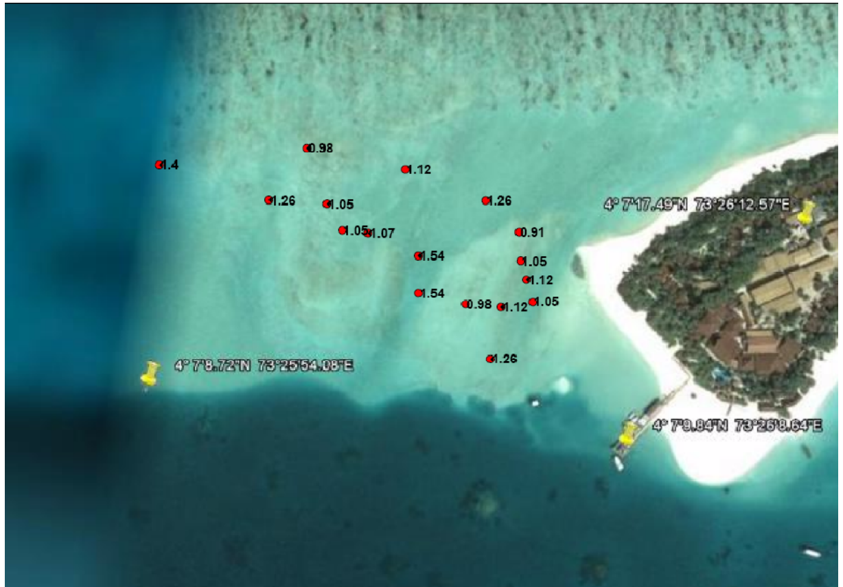
Figure 11. Shows the calculated maximum wave height in (m) that will be expected in the area proposed for overwater villa and spa complex development. The black dot marks the location of S4 current meter was deployed for current measurements.
