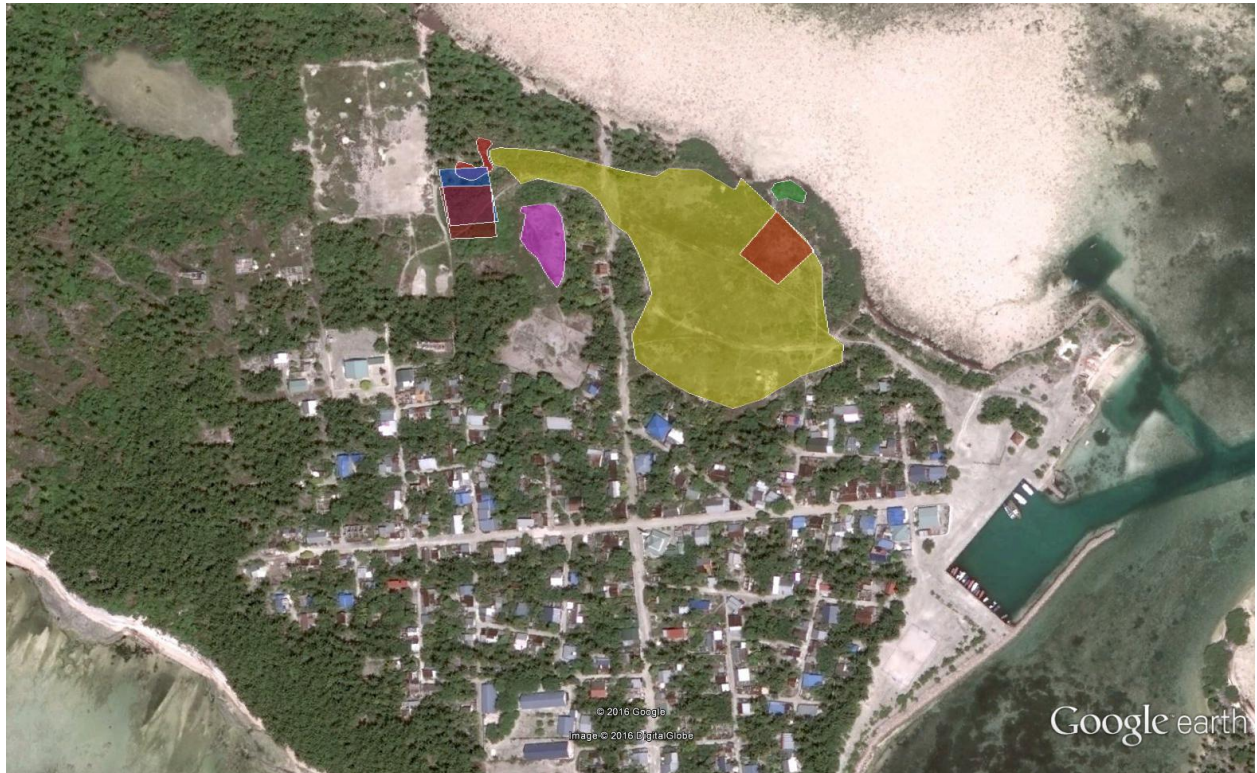
Figure 23: alternative location for powerhouse. In yellow is the reclaimed wetland area, maroon is the alternative location option 1, orange is alternative location option 2, red is the existing wetland, blue is the given plot for powerhouse, green is the waste disposal area, and purple is the graveyard.
