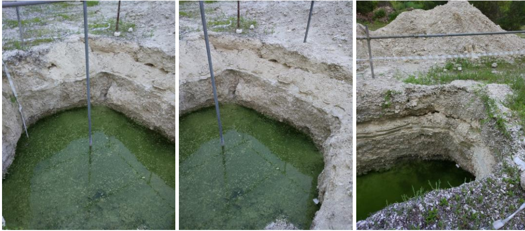
Figure 12 Groundwater collection pit including soil profile.
