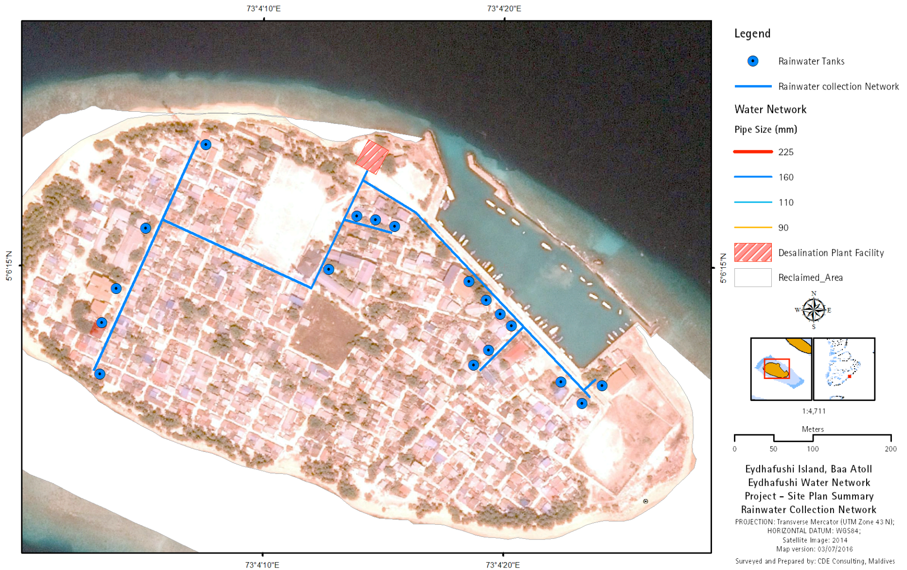
Figure 2.2: Project rainwater network site plan summary
