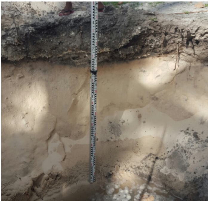
Figure 4.9 Baa Eydhafushi RO Plant Site Soil Profile
