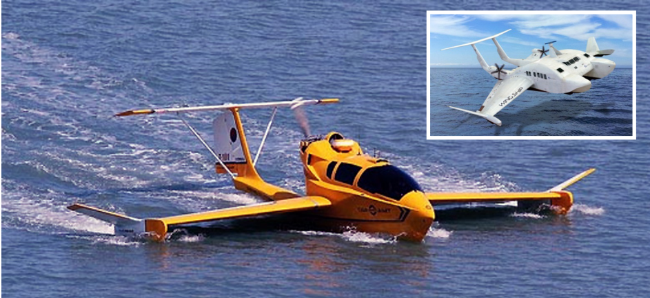
Figure 3. The Korean Aron-7 and WSF-50 (inset). South East Asia now leads in the development of WIG craft.
