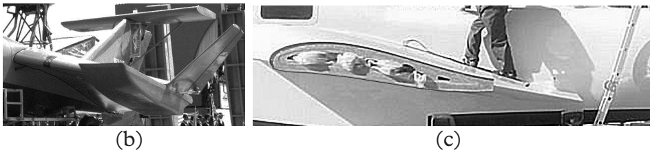
Figure 9. The airfoil (a) of a 20 seat WIG showing sandwich construction (Kong, Park, & Kang (2008)). The image (b) shows the photographically emphasized deep under-cambering of Bavar 2. The airfoil (c) is that of the Chinese craft seen in the Figure 6. It has been enlarged and flipped horizontally so that the orientation of the two images is the same.
