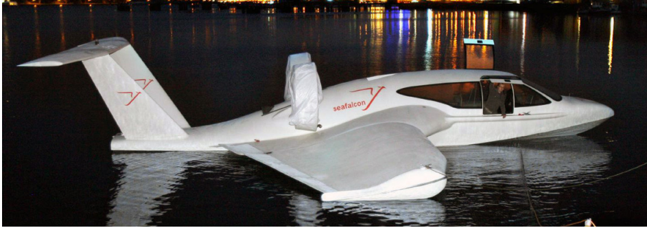
Figure 4. Seafalcon is made of glass-reinforced polymer.
