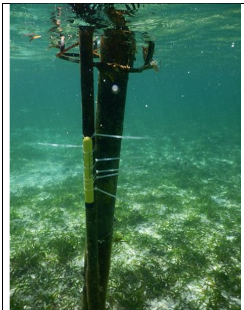
Figure 20: RBR Solo wave measurement device (Wave Gauge) deployed in shallow water
