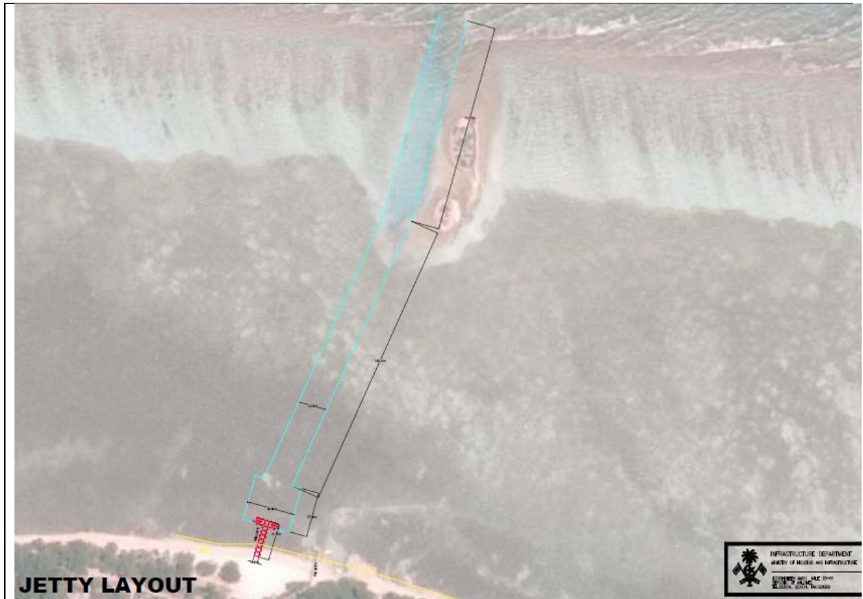
Figure 11: Conceptual drawing and location of the proposed access channel and jetty
