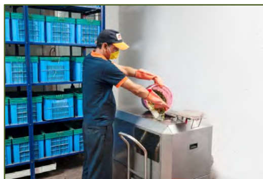
Pic 2: Input wet waste into OWC with Bioculum
