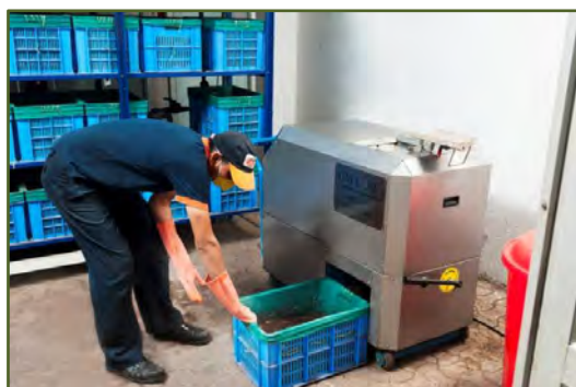
Pic 3: After 15 minutes collect raw compost from OWC
