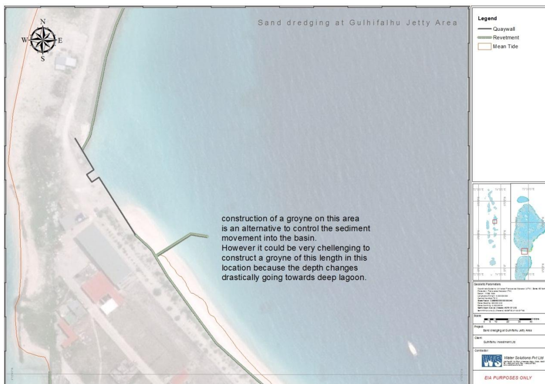
Figure 27: Alternative concept (A2): Construction of a groyne could provide temporary solution to basin filling problem
