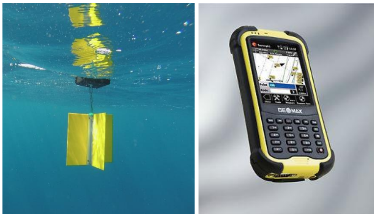
Figure 11. Drogue deployed at sea for current measurement (left) and hand-held GPS used to geo-reference sampling locations
