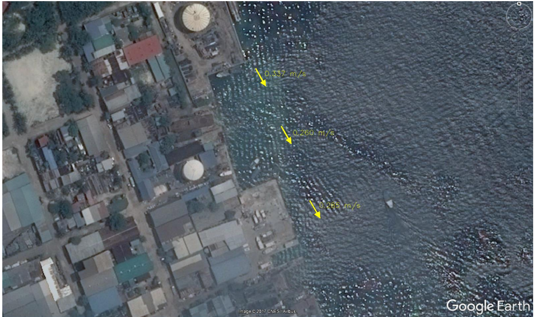
Figure 32. Current patterns on the Eastern side of Thilafushi
