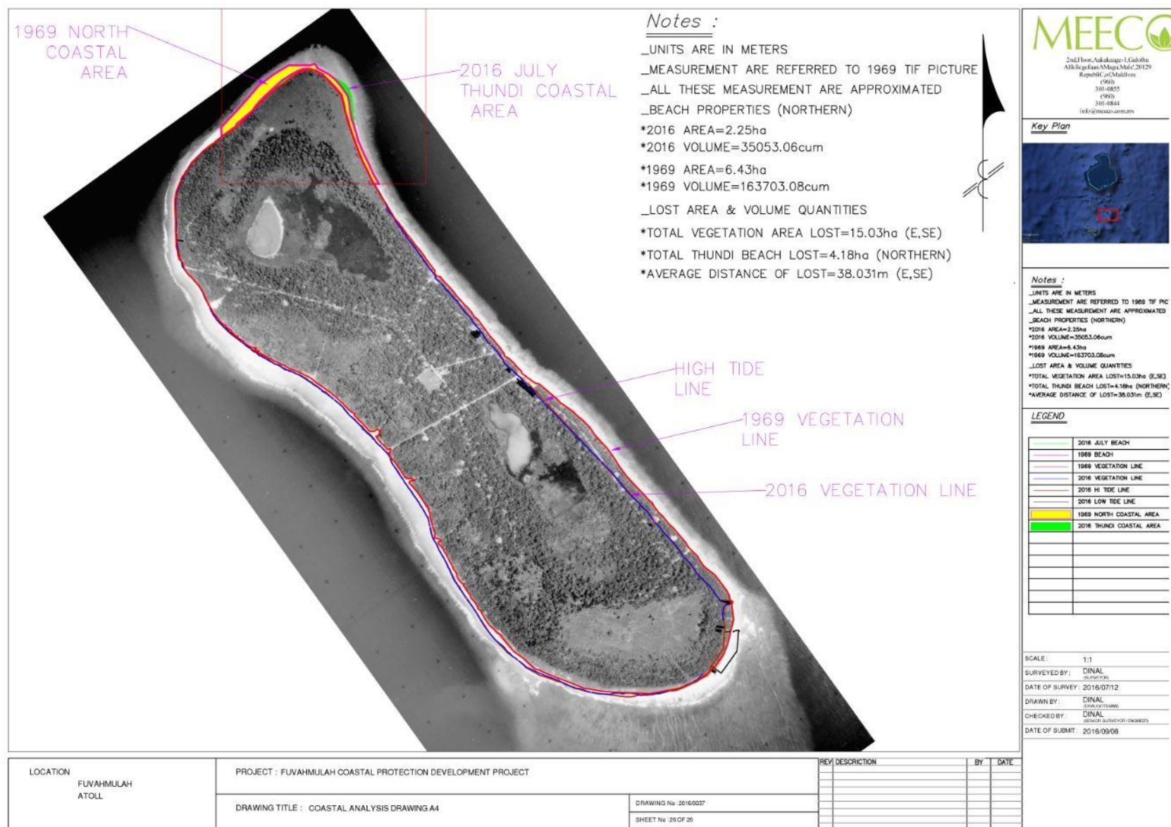
Figure 23: North-eastern shoreline erosion of Fuvahmulah from 1969 to 2016
