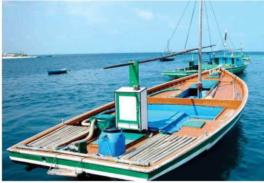
Figure 1.8: Second generation masdhoani. Specially designed wooden boat for pole and line fishing. There was not shelter.
