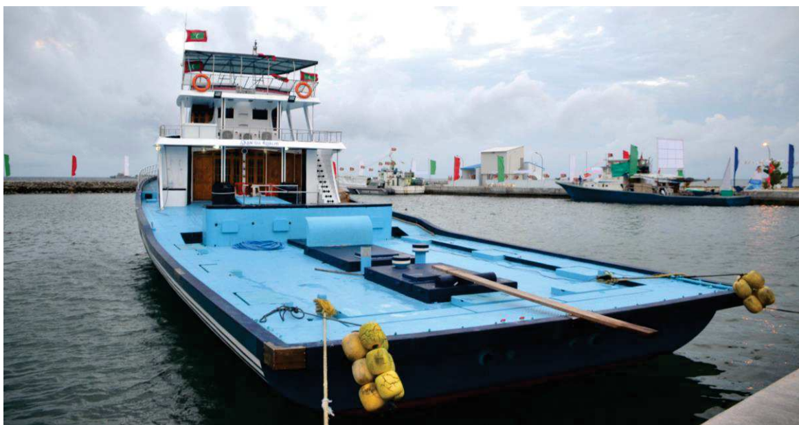
Figure 1.10: Present – modern fibreglass masdhoani widely used for tuna fishing across the Maldives.
