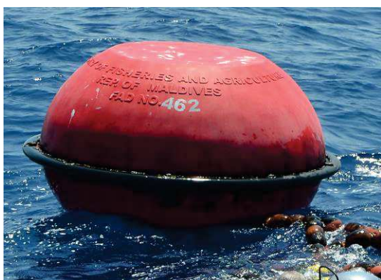
Figure 2.2: FRP buoy that serves as the float for the AFAD with the Ministry and country name embossed.
