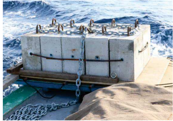
Figure 2.5: Three-ton anchor made from interlocking concrete blocks.
