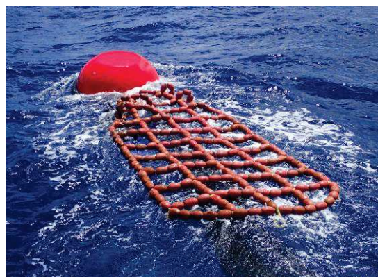
Figure 2.3: AFAD deployed at sea – main buoy and set of floats at the surface.
