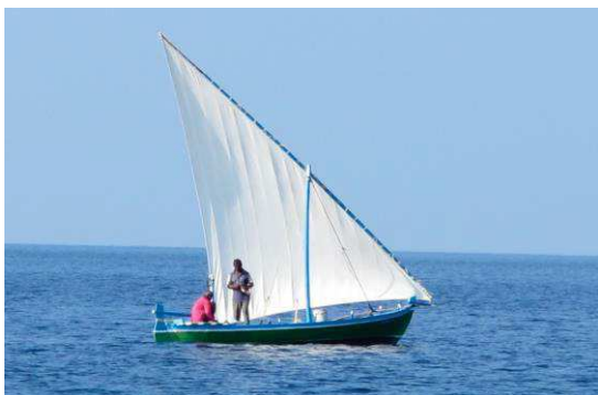
Figure 1.20: Traditional sailing trolling vessel.
