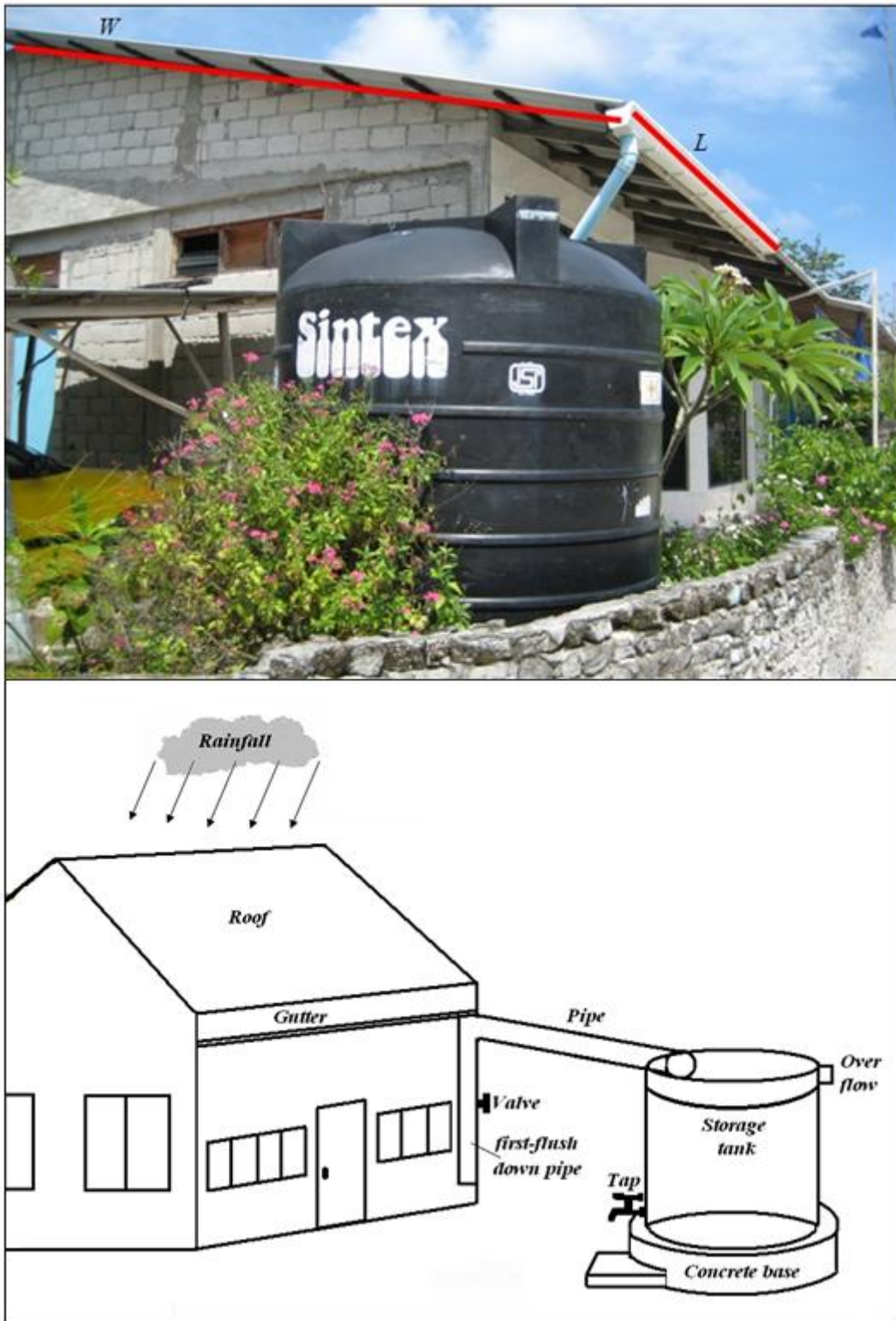
Figure 8.21: Actual (top) and schematic diagram (bottom) showing typical rainwater harvesting systems observed in the Maldives. Most of the households use only part of the roof (the gutter is only connected to a part of the roof) for harvesting rainwater.
