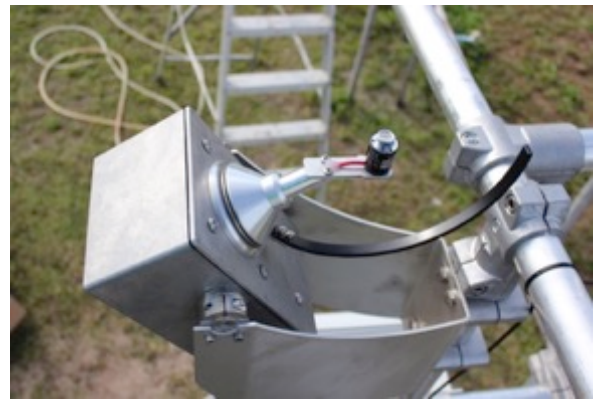
Figure 3-6: Rotating Shadowband Irradiometer - View from top
