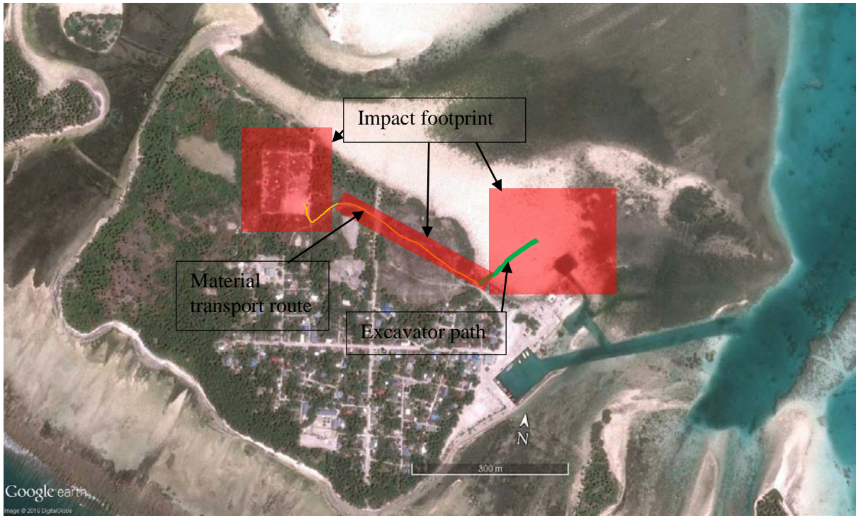
Figure 3: Project impact footprint, excavator path and material transport route
