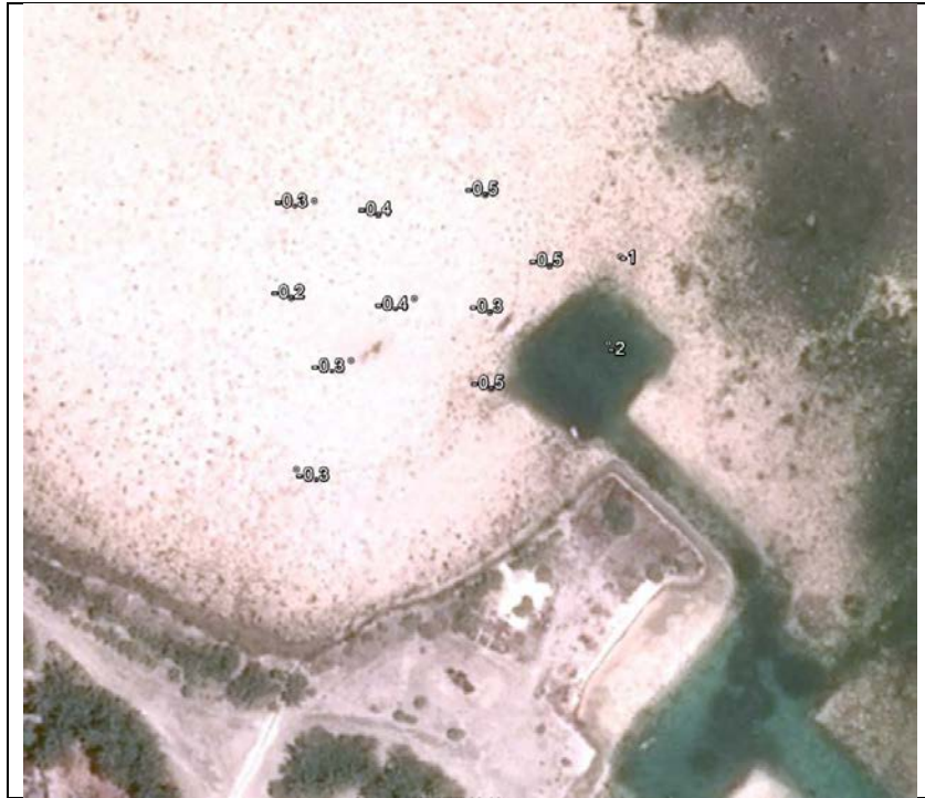
Figure 10: Nearshore depth around the area proposed for dredging.
