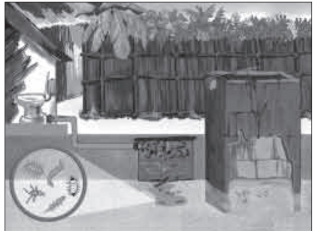
Well contamination from leaking septic system.
