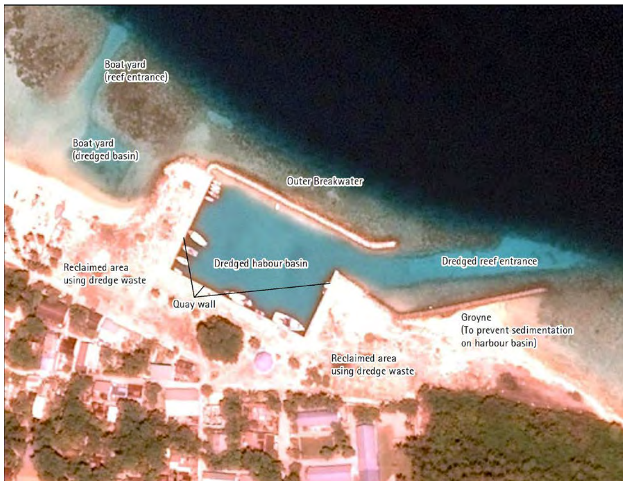
Figure 4.1 Basic elements of harbor infrastructure
