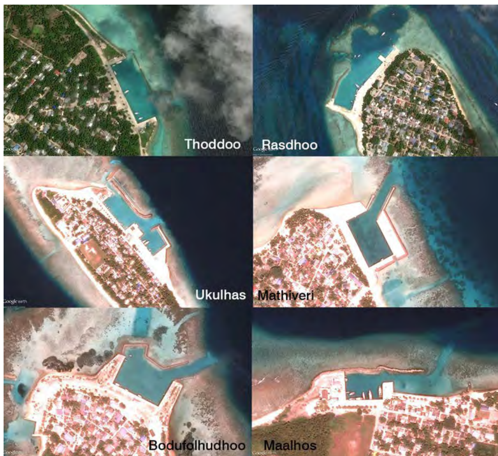
Figure 4.2 Harbour designs used in the inhabited islands of North Ari Atoll
