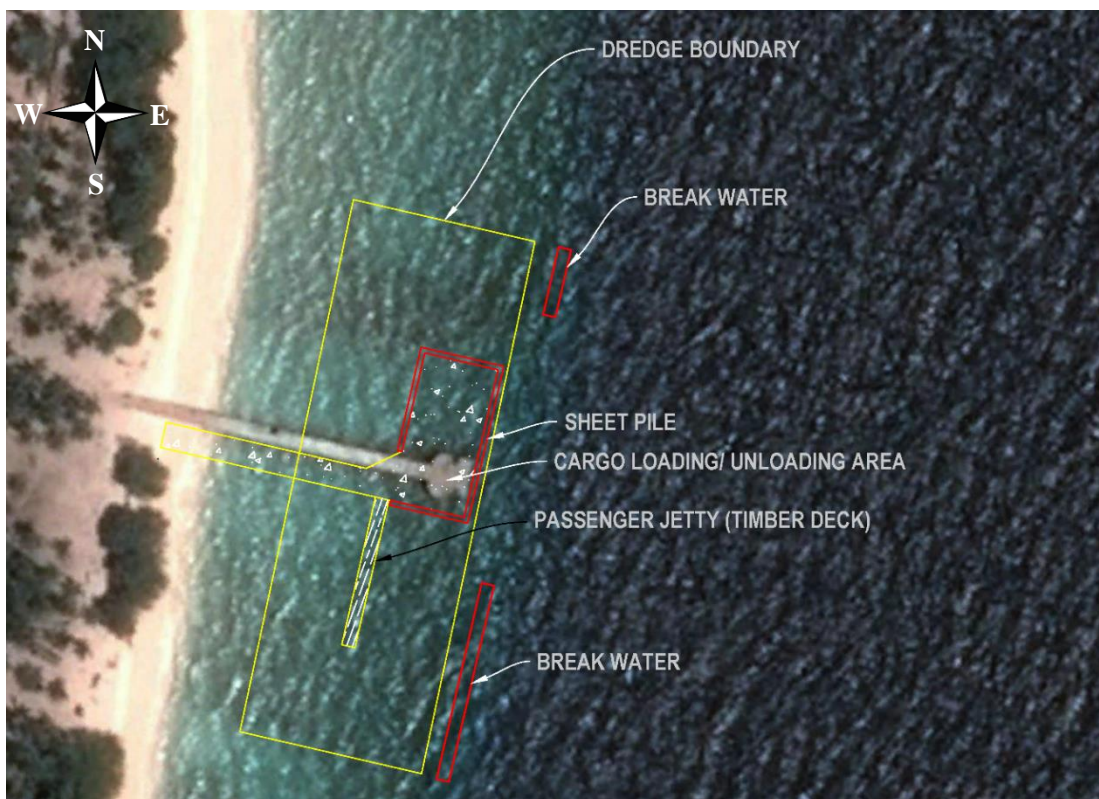
Figure 28. Proposed alternative design to ease berthing and to protective measures for shoreline and basin.
