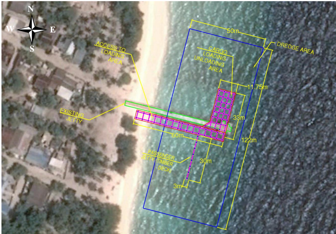
Figure 4. Design concept of the N. Fodhdhoo jetty.
