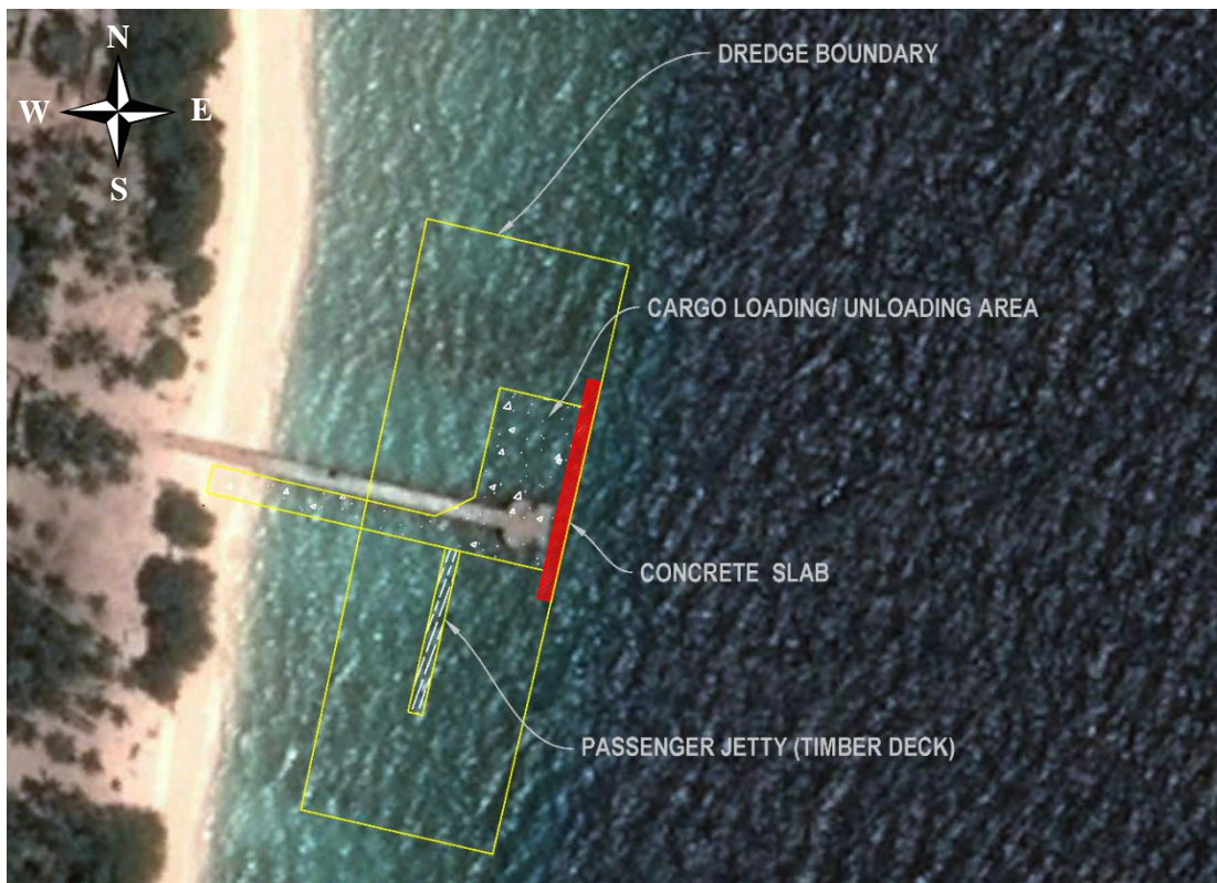
Figure 27. Proposed alternative design concept to ease access to jetty during rough conditions.
