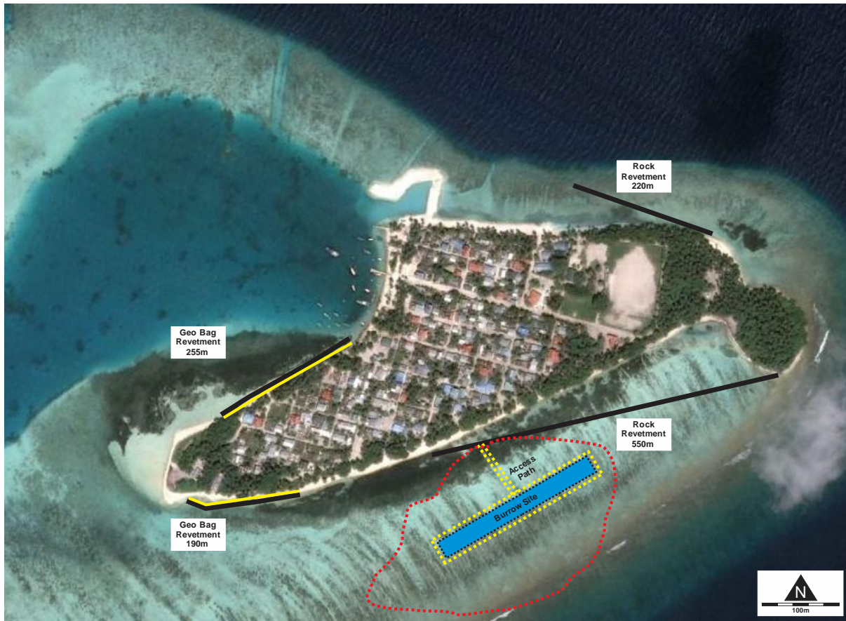
Figure 2: Impact boundaries of the new burrow site (yellow = activity area; red = anticipated impact boundary)
