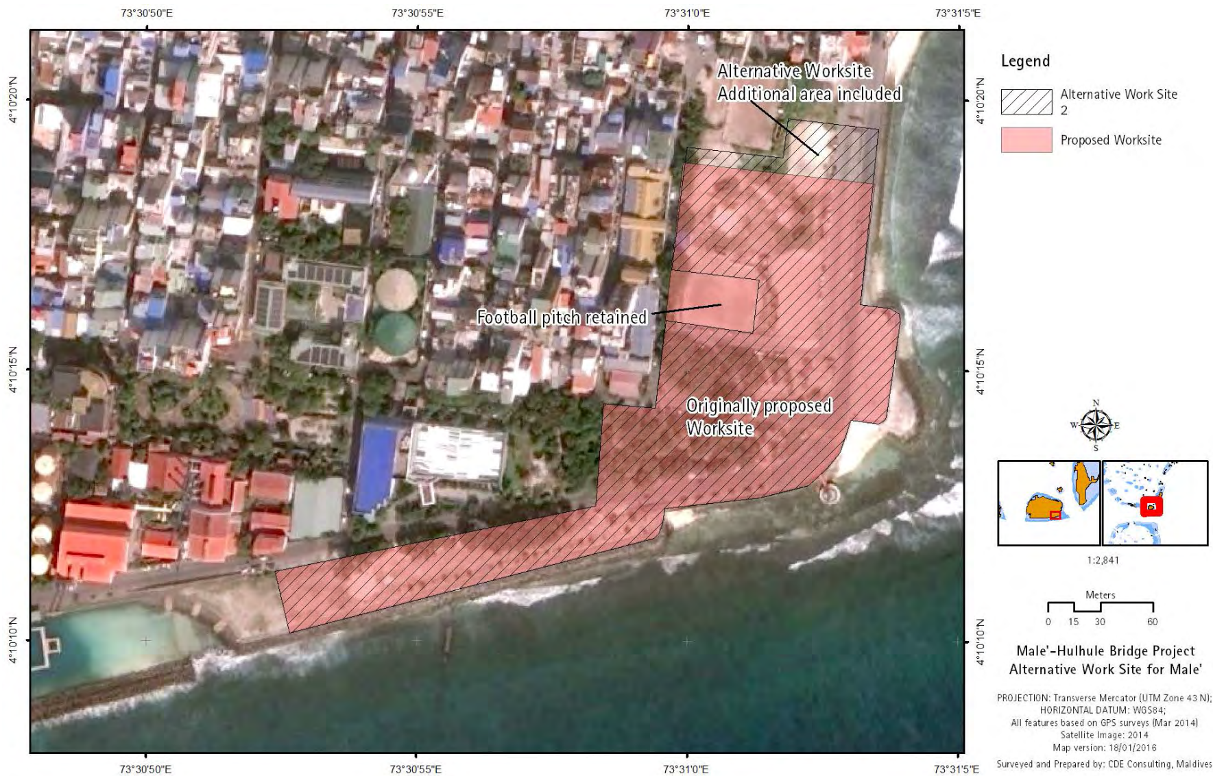
Figure 7.2: Alternative concrete batching plant sites
