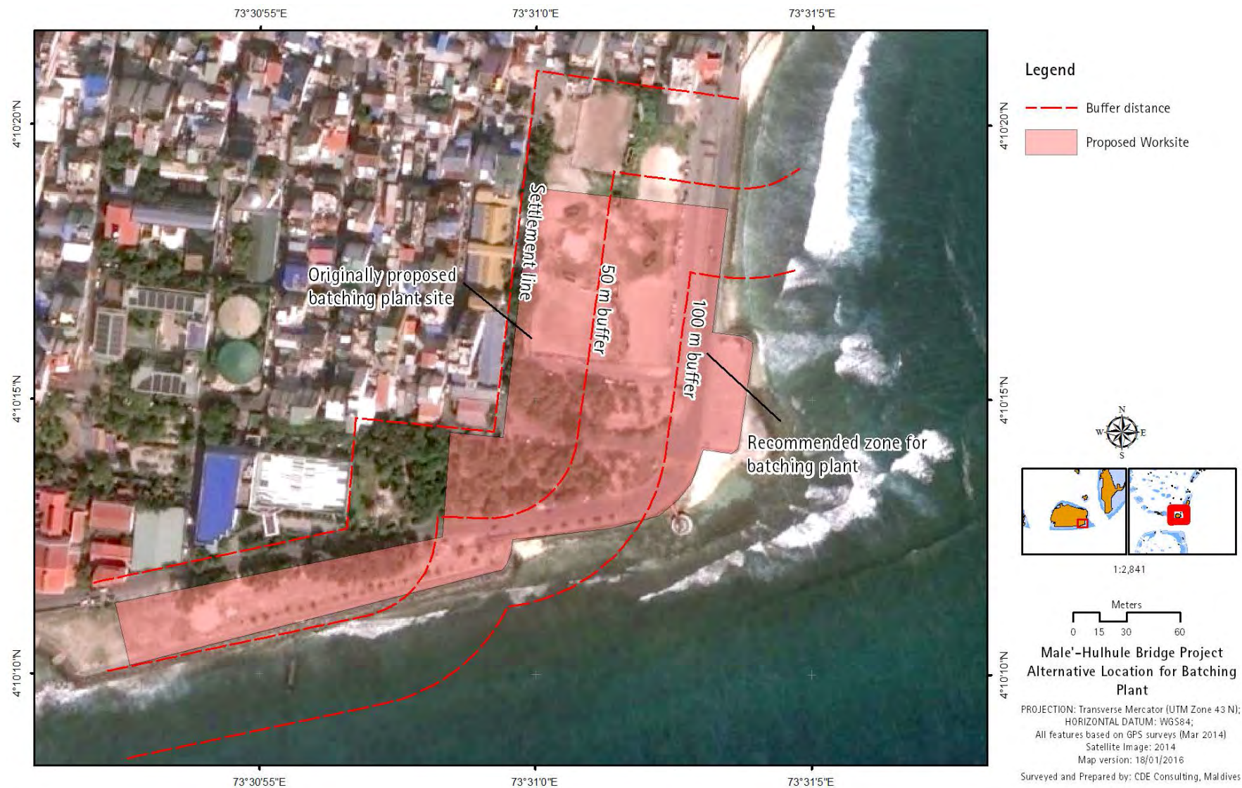
Figure 7.1: Alternative concrete batching plant sites
