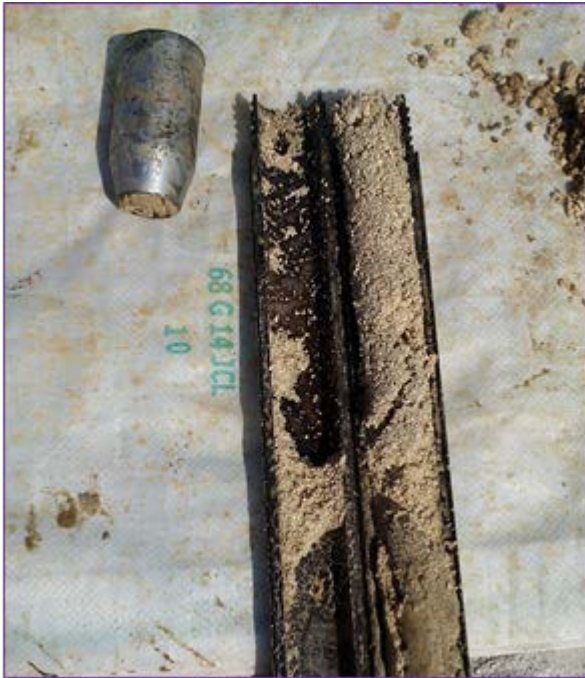
Figure 2.3: A view of Split barrel sampler with coral sand collected
