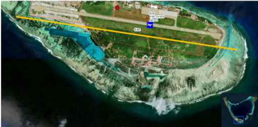
Figure 7: Map showing potential sites for the radar tower, at a minimum distance of 300m from the runway
