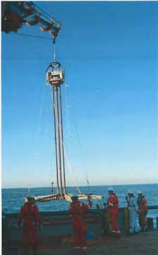
Figure 4. High power electric vibrocorer being deployed.
