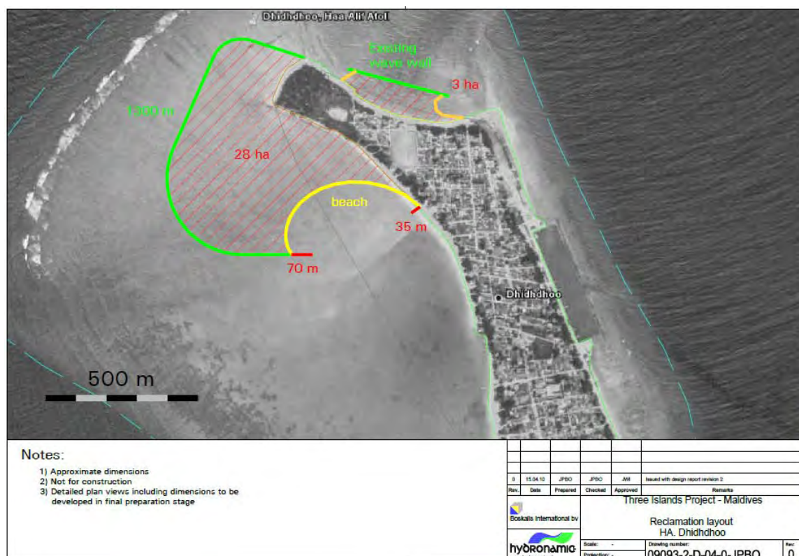
Figure 5-1 - Preliminary design of reclamation areas, revetments, beach and groynes at Dhidhdhoo
