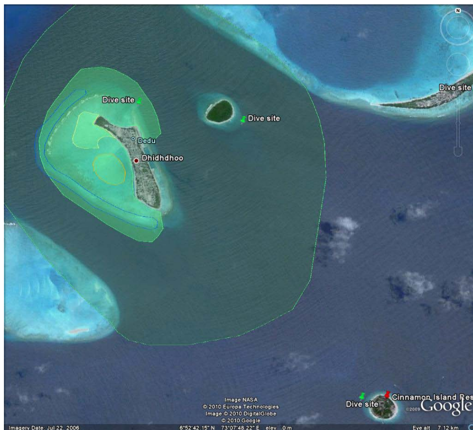
Figure 9-1 - Possible area of direct influence (bright green, temporary increase in suspended sediment concentration during dredging and reclamation works) and less direct influence (darker green, short term reduction of visibility during storm events) of suspended solids released from the proposed borrow area and the reclamation area under worst case conditions
