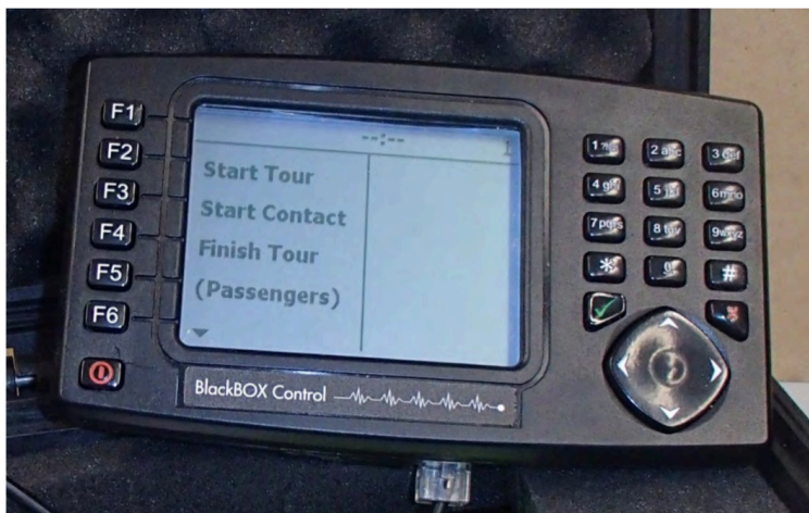
Figure 14: The electronic GPS based log book system (EMS) (source: Department of Parks and Wildlife, 2013, p. 22).
