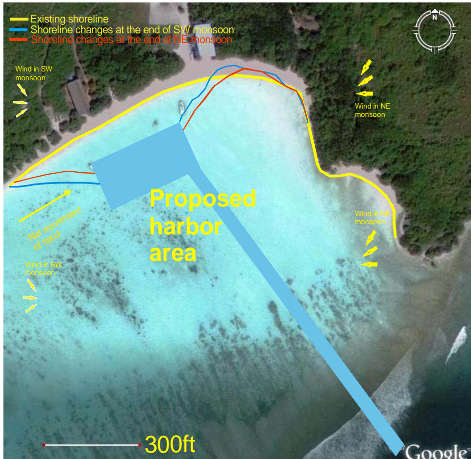
Figure 15: Possible alteration of shoreline as a result of harbor construction
