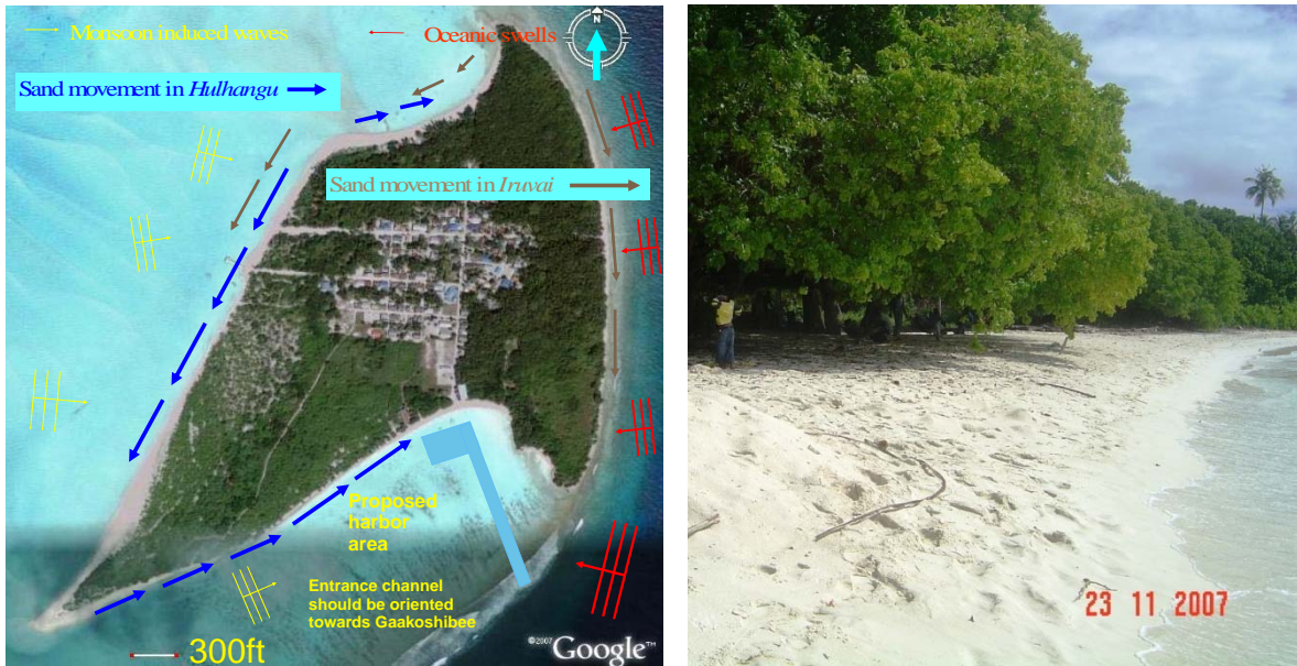
Figure 7: Wave and sand movement around Bilehahi during the two monsoons (left). Fine grained sand at the proposed harbor area (right).
