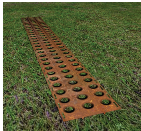
Figure 3: Marston Mat, more properly called pierced (or perforated) steel plating (PSP), is standardized, perforated steel matting material developed by the United States at the Waterways Experiment Station shortly before World War II, primarily for the rapid construction of temporary runways and landing strips (also misspelled as Marsden matting). The nickname came from Marston, North Carolina, adjacent to Camp Mackall airfield where the material was first used. (Source Wikipedia)
